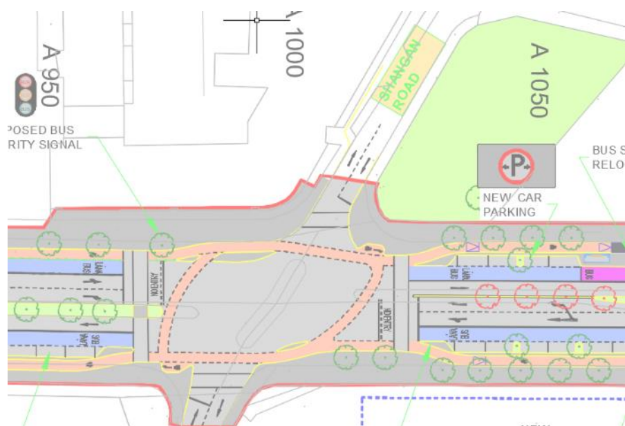
Figure 2-1 Junction Type 1 Proposed Shangan Road Junction
